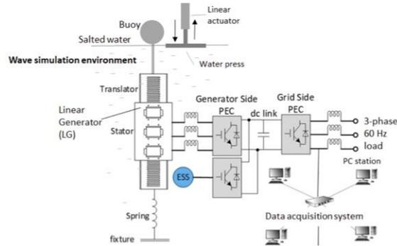
Fig. 1. Schematics of the proposed integrated wind and wave energy laboratory
