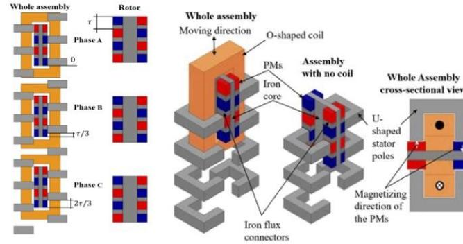
Fig. 2. Direct-drive transverse-flux linear generator for wave energy conversion
