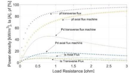
Fig. 7. Steady-state characteristics of the transverse flux generator compared to the conventional axial flux generator
