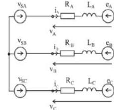
Fig. 6. Equivalent circuit of the generator
