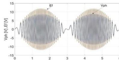
Fig. 5. Induced voltage of the generator at sinusoidal speed of the buoy
